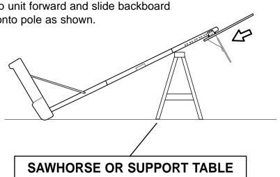
Attach board assembly to pole with carriage bolts (16) and knobs (11) as shown. Install pole cap (7) as shown.
